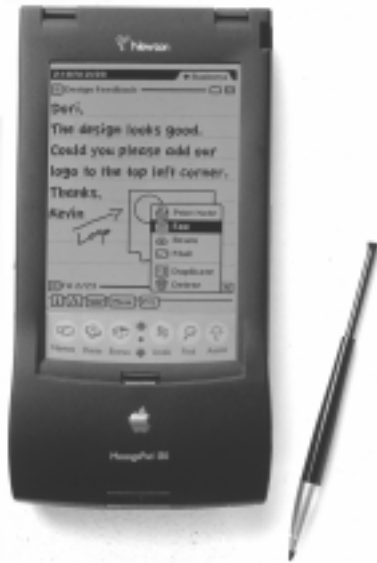
The MessagePad 130 was the first Newton to come with a backlit screen.
