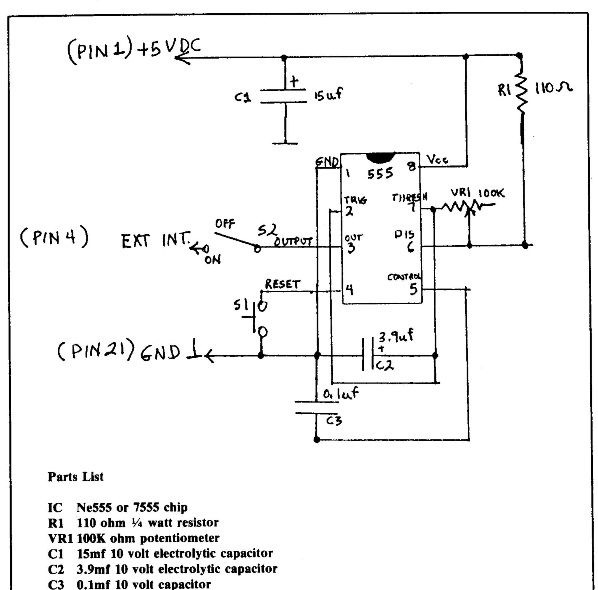
timing circuit to determine the delay prior to the 555 flip-flopping. Capacitor C3 provides a reference voltage for the control gate. Switch S1 places the reset pin low when pressed and causes the output to go low thereby generating an interrupt. Switch S2 connects the timer to the interrupt pin of the computer. The timer circuit operates whether or not it is connected.
