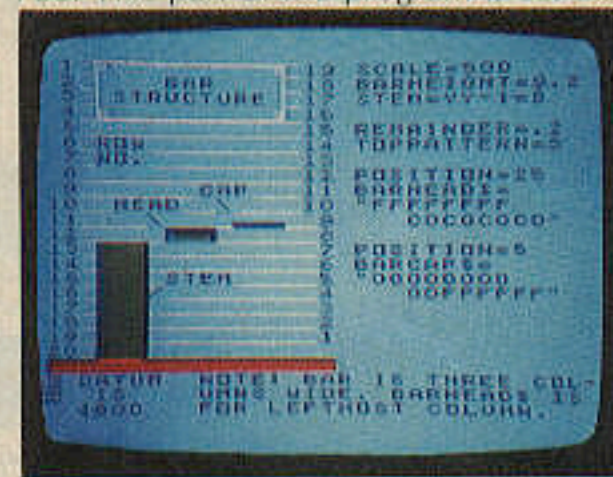
Figure 3. The three parts of a bar involved in the outlining routine. With this example, three pixel rows will be turned on in the bar cap, and in the bar head the top four pixel rows will be black.
