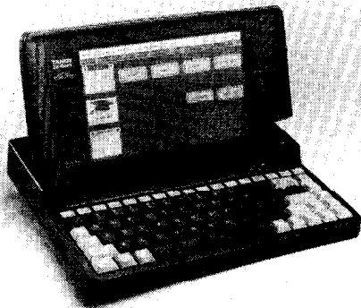
The new Tandy 2810 HD includes a built-in hard drive, floppy drive, MS-DOS 4.01, and DeskMate.
