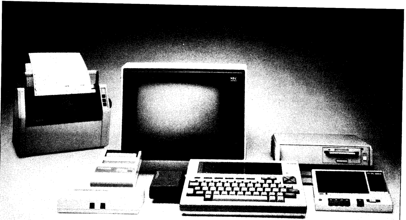
Peripherals available for the NEC PC-8201A from NEC Home Electronics — Two portable printers: 80-column width and 40-column width, cassette tape recorder, monochrome monitor, an additional RAM bank (32K), micro-floppy diskdrive, and 300-baud modem.
