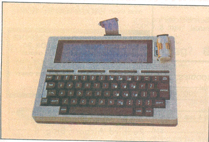
Photo 1. Model 100 with two AA batteries taped next to the display.
