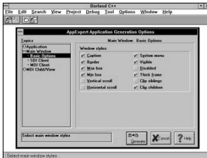
Figure X3.7. The AppExpert dialog box showing the Basic Options subtopic in the Main Window topic.
