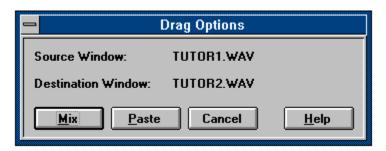
5 Press either the Mix or Paste buttons to finish the operation or press Cancel to skip the operation.
