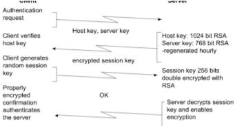
The client generates a 256 bit random number using a cryptographically strong random number generator, and chooses an encryption algorithm from those supported by the server, normally Blowfish or three-key triple-DES (3DES). The client encrypts the random number (session key) with RSA using both the host key and the server key, and sends the encrypted key to the server.
