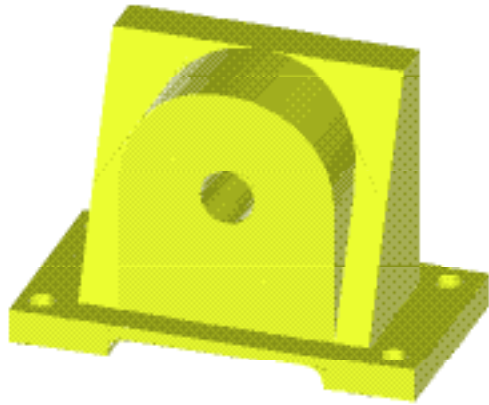
Figure 11-6. This part was made using the Solid Subtract and Solid Add commands
