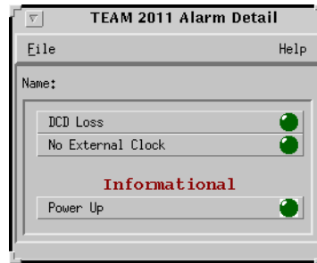
Figure 2-2 Alarm Detail Window
