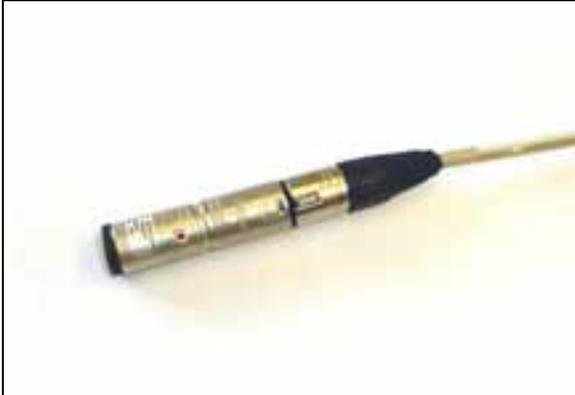
The FinishLynx Start Sensor detects the changes in air pressure caused by the firing of the gun and sends a signal to the computer. FinishLynx will operate with a variety of start signal generators.
