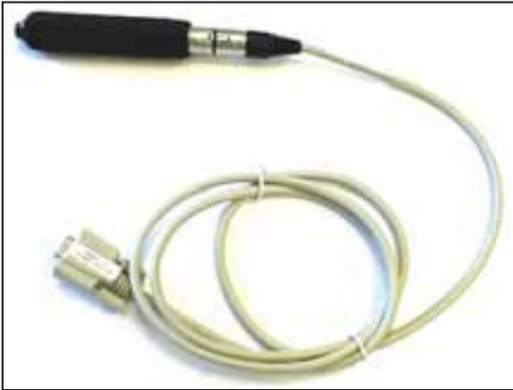
The Capture Button needs to be connected to a serial port on the back of your computer with the cable supplied.
