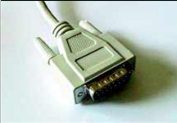
The DB15 connectors on the ends of the Connection Box cable are connected between the back of the Camera and the Connection Box.
