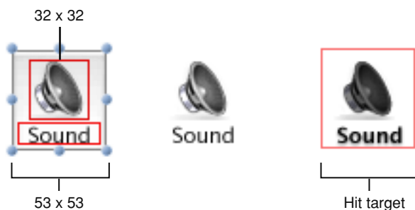
Figure 15-11 Example relationships of the icon, button, and hit-target dimensions in an icon button
