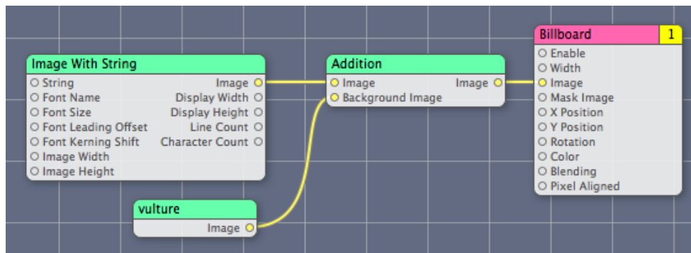
Figure 2-6 The Addition patch is a Composite patch
