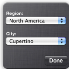
Figure 28 The Done button is a glass-style button, which is intended for use on a widget's back
