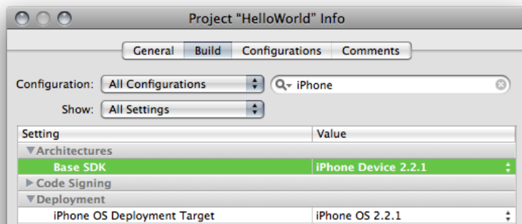
Figure 3-4 Base SDK and iPhone Deployment Target build settings
