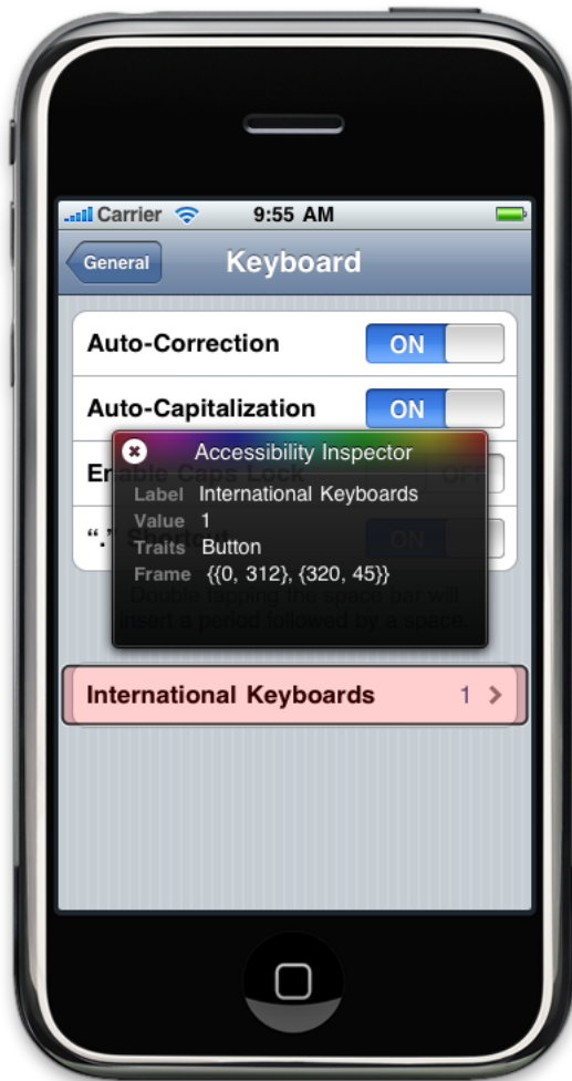
Figure 3-2 Accessibility Inspector draws a rectangle around the selected element
