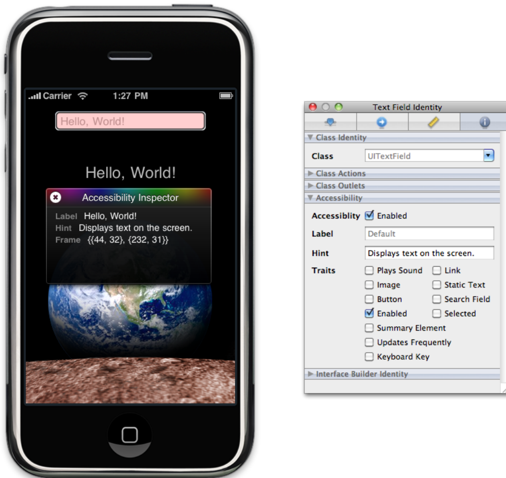
Figure 2-2 Supplying accessibility information in Interface Builder
