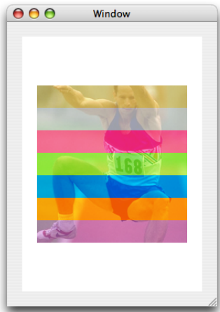
Figure 11-26 Drawing an image over a background using soft light blend mode
