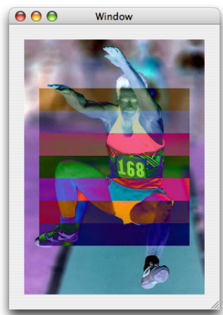
Figure 11-28 Drawing an image over a background using difference blend mode
