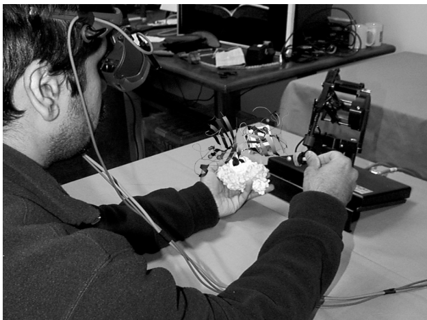
Fig. 7 User interacting with SOD model using HMD and PHANToM™. Virtual overlay shows SOD secondary structure and force fields.
