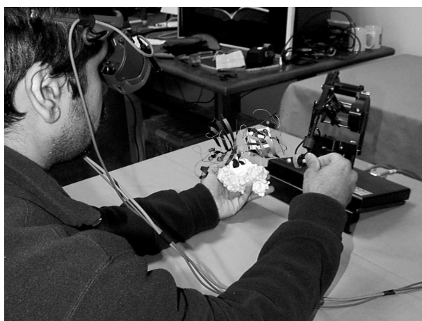
Figure 4. User interacting with SOD model using HMD and PHANTOM. Virtual overlay shows SOD secondary structure and force fields.
