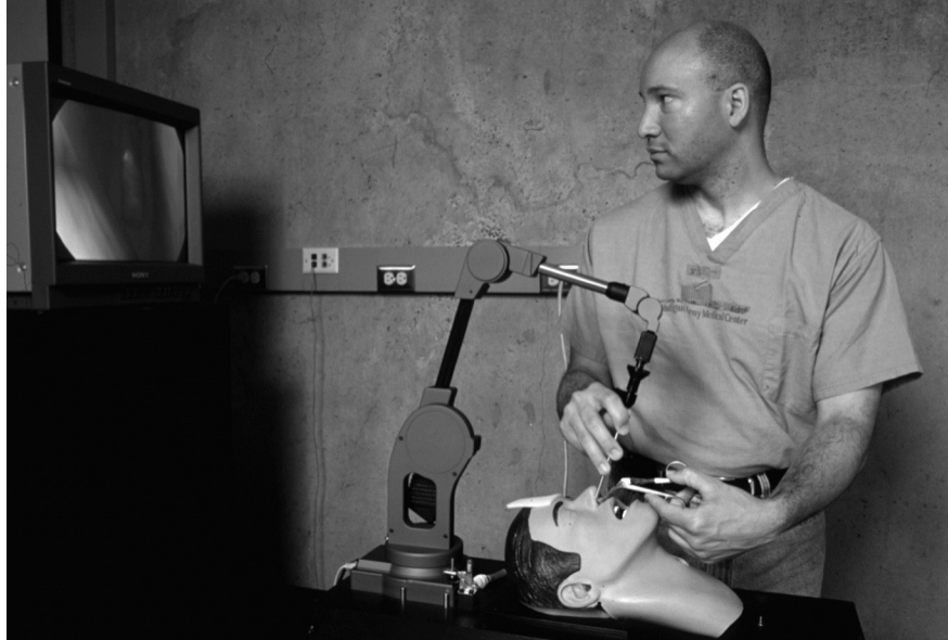
Figure 1. Operative configuration of the Madigan Endoscopic Sinus Surgery Simulator.
