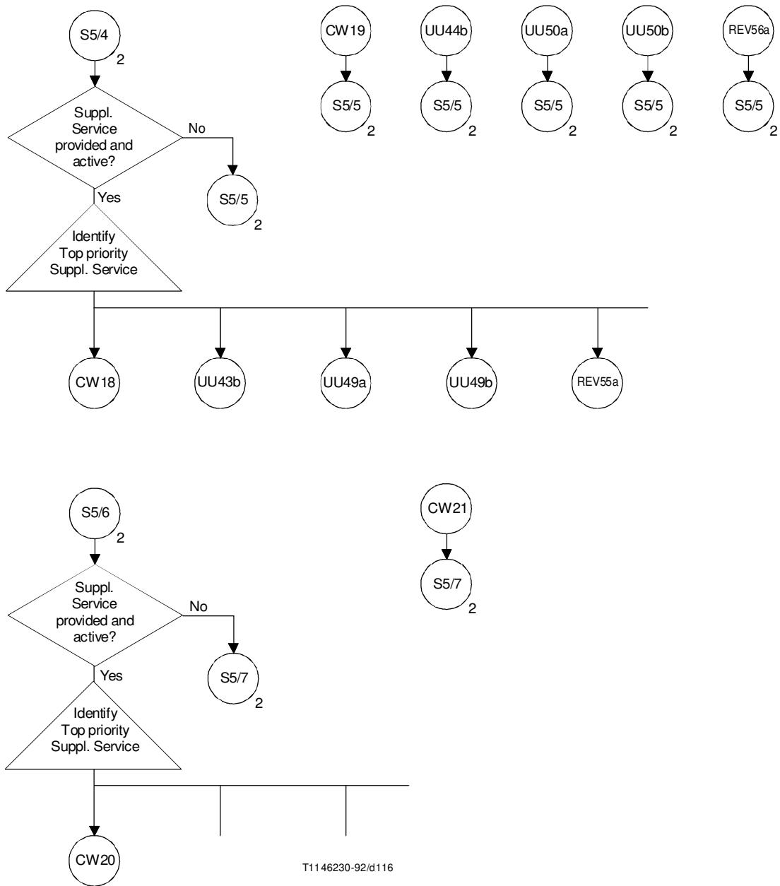
FIGURE A.5/Q.71 (sheet 6 of 12) CC (FE5) – Interworking with Supplementary Services
