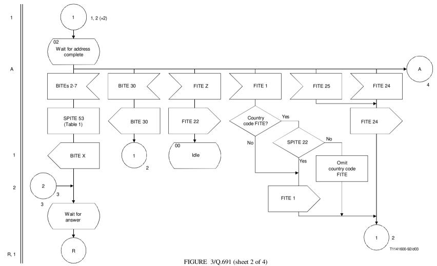
Interworking of Signalling System No. 7 (ISUP) to No. 6
