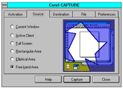
Corel Capture is a screen capture utility that saves areas of your screen as a BMP, CPT, or TIF file. Using a defined hotkey, it triggers a timed capture and saves it as a file. As with the other applications, a variety of options are available from the tabbed dialog, including the automatic generation of filenames.
