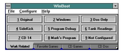
When started, the *WinBoot 2.0* utility presents a dialog box with a series of nine buttons. Each of these can be configured and named to suit the specific combinations of AUTOEXEC.BAT and CONFIG.SYS files you require for each specific setup. The buttons may be named anything you wish, but something more descriptive of the applications involved would probably work best.
