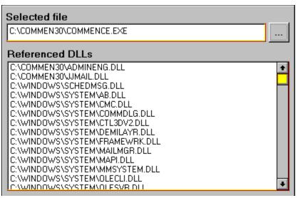
Want to find out which DLL and VBX files are being called by a particular application, to aid in an uninstall or diagnoses? Zero in on the file and let SCAN4DLL.ZIP (37K) do its work, returning a list that Wolly wishes he could print, or at least copy. He won't complain too loudly, 'cause after all, it's freeware from Software Innovations.
