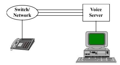
The fourth model, illustrated below, also works over the network, but instead of voice paths between the switch and the server, there is only a control channel. Thus, it can be used to set up calls and exploit basic network features, but it will not support applications like conferencing, voice annotation or anything else that uses the information carried on the voice path.
