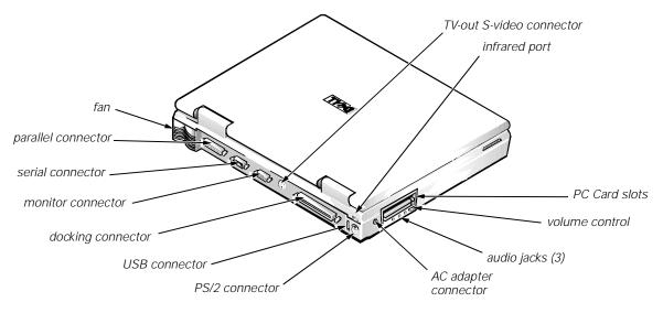
Figure 1-2. Back View of the Portable Computer
