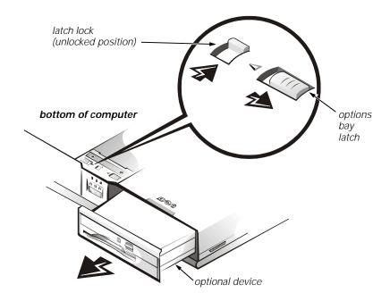
Figure 3-3. Checking an Optional Device
