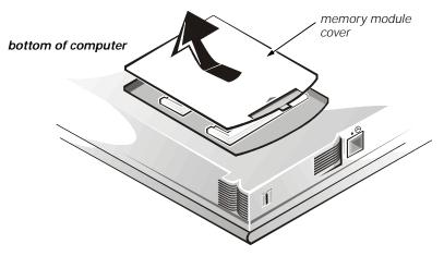
Figure 3-6. Removing the Memory Module Cover
