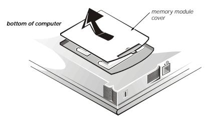
Figure 3-7. Removing the Memory Module Cover
