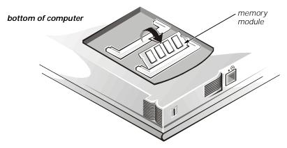
Figure 3-8. Removing a Memory Module
