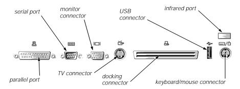
Figure 3-4. I/O Panel Connectors for External Devices
