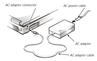
Figure 3-1. AC Adapter and Power Cable
