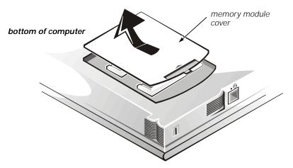
Figure 3-5. Removing the Memory Module Cover
