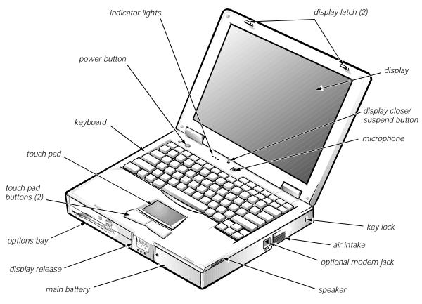
Figure 1-1. Front View of the Portable Computer
