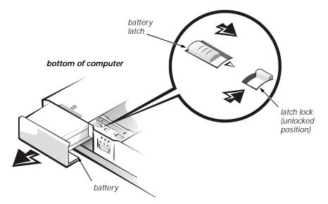
Figure 3-2. Checking the Battery
