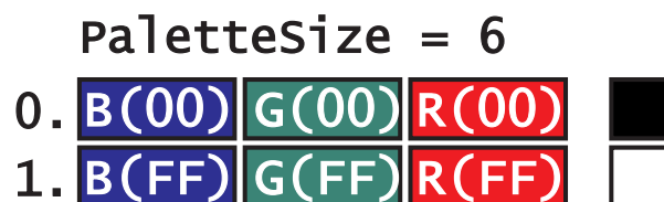
Figure 108. Palette Structure of a Black & White, One-Bit Image
