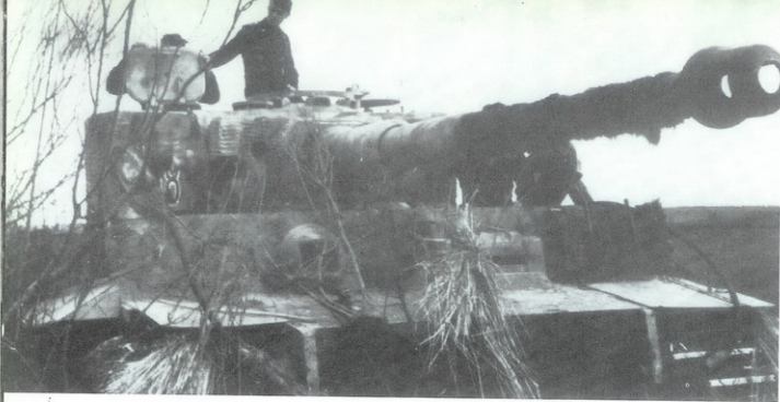
A Tiger with the new-type commander's cupola – the cover has been opened and can be seen at right by the ring for the anti-aircraft machine gun. Many Tigers – including this one – had towing cables hooked on during combat. (BA)
