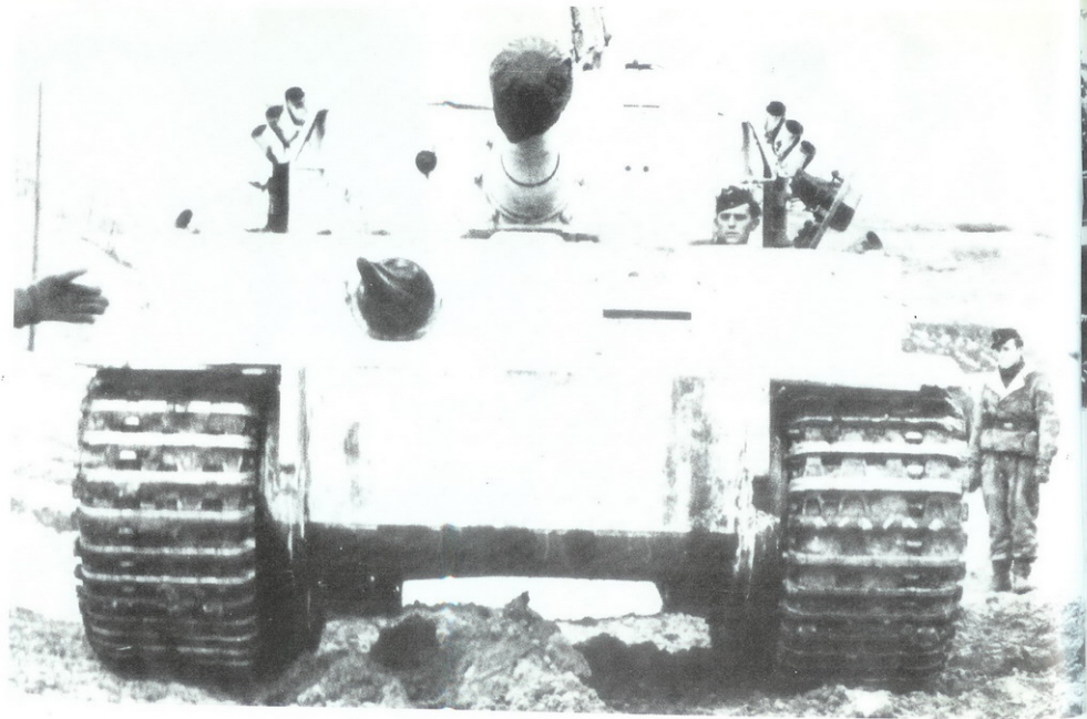
A well-camouflaged Tiger. Its tracks were 72.5 cm wide. By the launchers on the hull, the lack of reinforcement by the optics, and the commander's cupola, this is an earlier Tiger. (BA)
