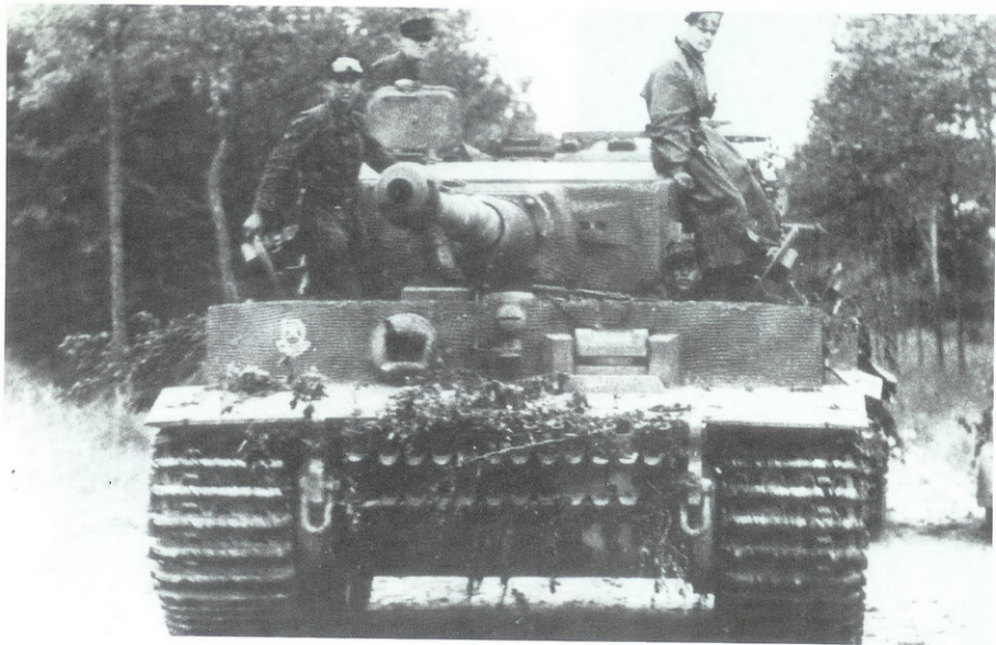
This tiger (newer type with flat commander's cupola) also shows the reinforced optical openings. By the emblem (two keys crossed) on the front, it belongs to the "Leibstandarte Adolf Hitler (LAH)" 1st SS Panzer Division. Unlike the previous Tigers, it has only one camouflage light, mounted centrally – the earlier type had one on each corner of the hull. (BA)
