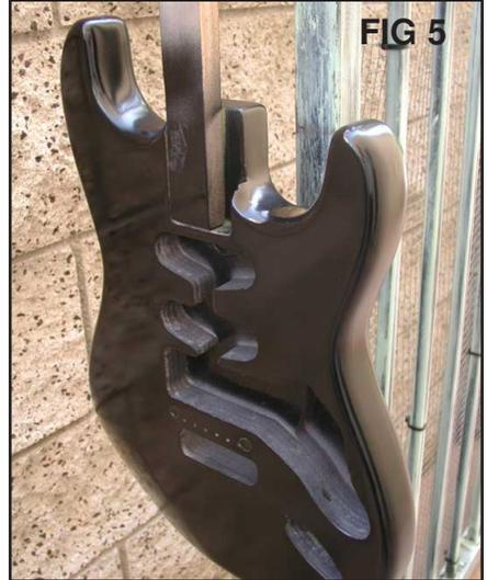
I very seldom ever get a run when using spray cans because I make sure I don't overdo it on each coat. However, when I do get a run, I hold the body in a horizontal position for a few minutes to help the paint even out. Try this for yourself if you experience a run or two.
