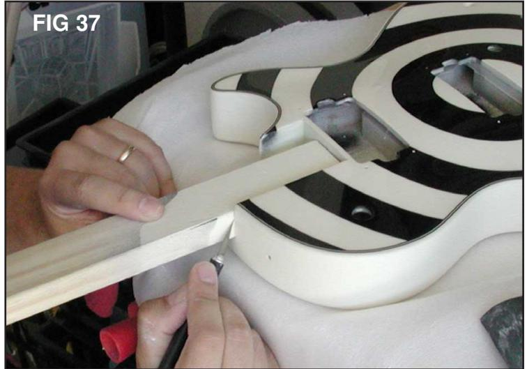
Go over it a few times so that when you remove the screws and stick, it separates easily from the body.
