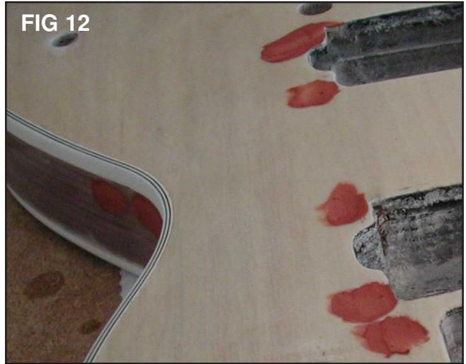
*For Project EVH, I didn't have to use any Bondo to fill the holes, so I'm using the photo from Project ZW as an example. I applied the Bondo with my finger, but I'd recommend that you apply it using a scraper. Simply squeeze the Bondo onto the scraper and press the Bondo into the holes. Scrape off any excess.*
