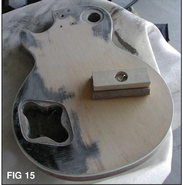
If you can carefully keep the sanding sealer that's already on the body, this will save you a considerable amount of time in the prepping stage, as it will eliminate the step where you'll have to apply sanding sealer to seal the body and get rid of the grain of the wood.
