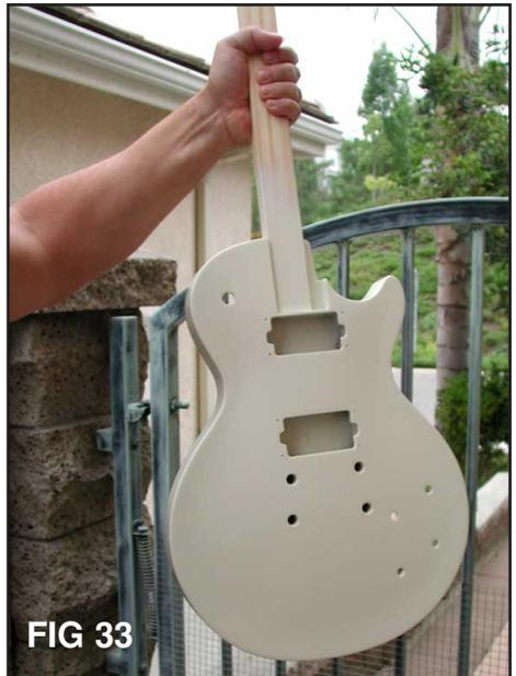
*Here I am holding the Project ZW body after the final coat of Ivory Gloss has dried. The body has the standard "orange peel" look, but otherwise, it's relatively smooth with absolutely no runs.*
