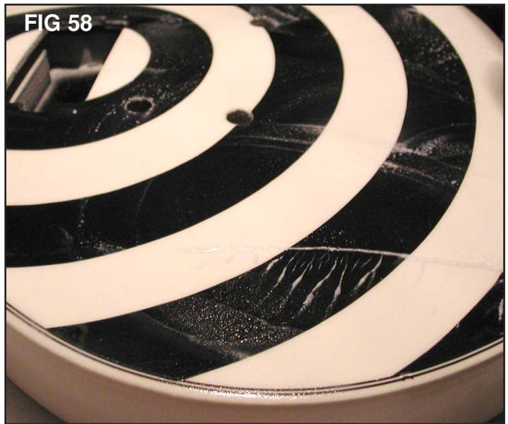
Be very careful when sanding on the edges of the body. In fact, I recommend you don't sand them with anything heavier than the 600-grit. It's extremely easy to go through to the paint and primer and right to the wood when sanding on the edges. Because it's an edge, paint just doesn't get built up the way it does on other parts of the body. **BE VERY CAREFUL WHEN SANDING ON OR CLOSE TO THE EDGES.**
