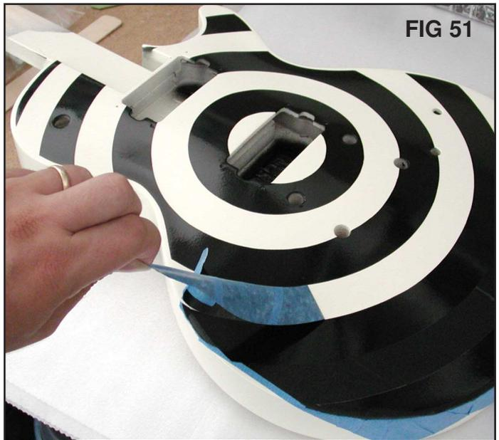
If, after all of the tape has been removed from the top, you notice that you'll need to touch up a couple of the lines, leave the masking tape on the sides and back until all touch-ups on the top have been done.
