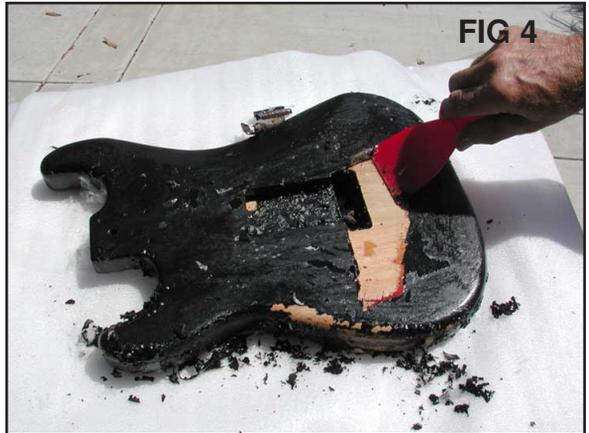
*This photo shows how good the paint stripper works - the finish is coming right off in sheets.*
