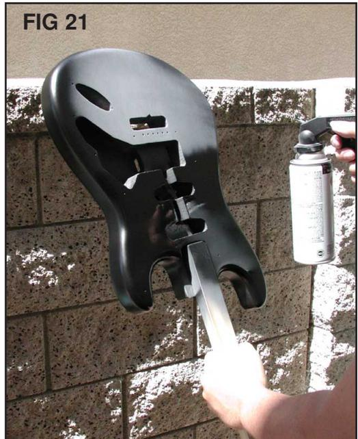
*Here I man applying my first coat of color in a "left to right, right to left" manner. I sprayed the sides first, which is why you see paint around the edges.*
