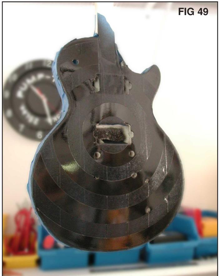
When you've completed the necessary coats, let the body sit for a few hours before proceeding to the next step - Removing The Remaining Masking Tape.
