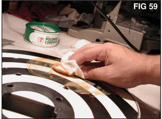
*I initially started using a different rubbing compound than the one I recommend you use. I quickly switched to the 3M Perfect-It II when I didn't like what this compound was doing to the surface. You can see in this picture that I work in an area of about 4" x 4" at a time.*
