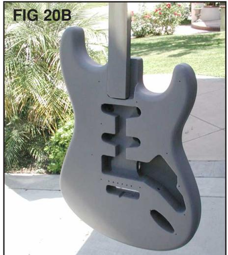
*Here's the finished body, sealed, primed, and ready for its first coat of paint.*
