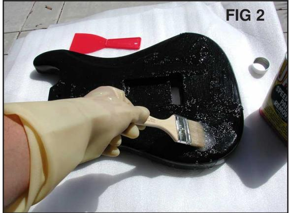
*The benefit to using styrofoam under your guitar body when using paint stripper is that the styrofoam will not melt.*
