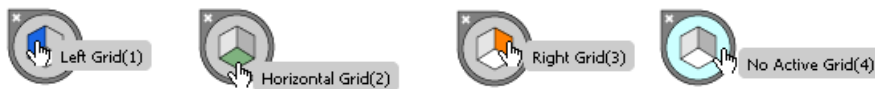
Figures 2.13a and 2.13b Changing the active plane in a grid using the Plane Switching widget.
