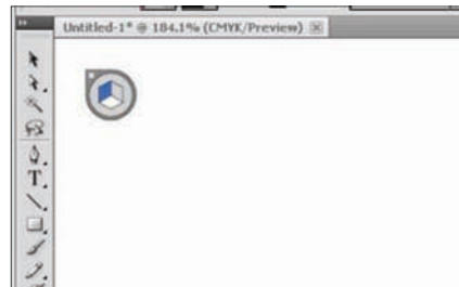
Figure 2.12 The icon indicates that the left vertical plane is active in the Perspective Grid.
