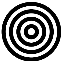
Figure 15.12 The diffraction produced by a single circular aperture consists of concentric light and dark bands.
