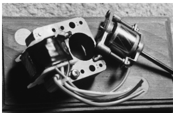
Photo 25.5 AC induction motor.
