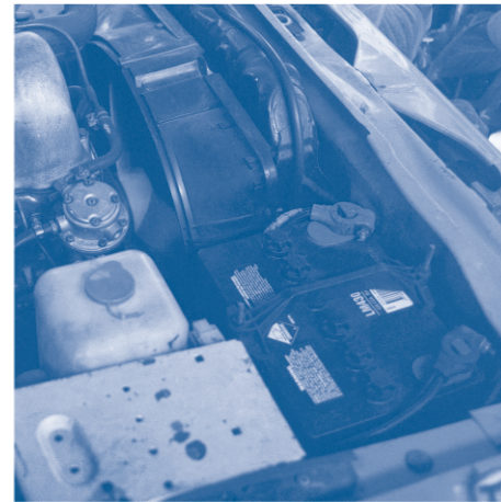
Photo 22.1 The battery in a car.
