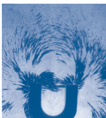
Figure 25.6 Lines of magnetic field (lines of flux).
