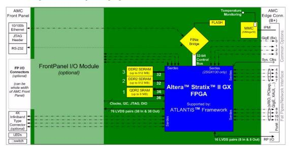
one bank of QDR2 SRAM, and Flash memory for booting the FPGA and FINe.
