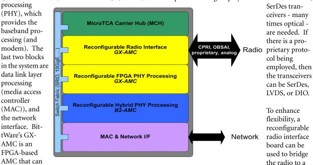
be used for both the radio interface and the physical layer processing. If a DSP is required, BittWare's hybrid signal processing AMC - the B2-AMC - can be used for the PHY processing. Both boards provide a reconfigurable interface that can be tailored to the required task.
