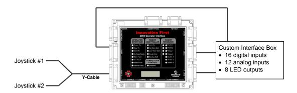
Figure 4.3.3: Operator Interface with Two Y-Cable Joysticks and a User Box
