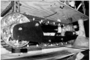
Studs in tread help keep tread from derailing
