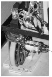
This compand drive/steering mechanism allowed the vehicle to move in any direction from a stopped position (zero turning radius)
