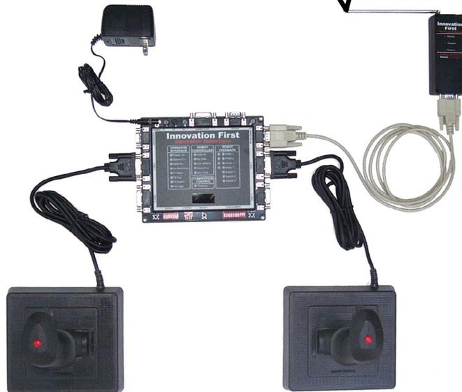
Operator Interface with External Radio,
