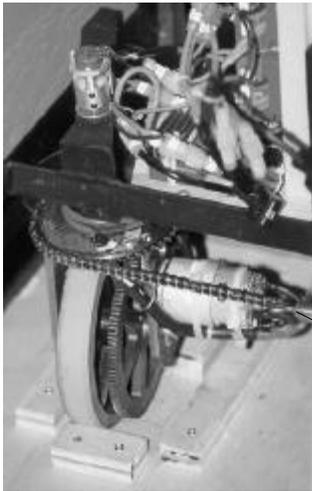
This compound drive/steering mechanism allowed the vehicle to move in any direction from a stopped position (zero turning radius)
