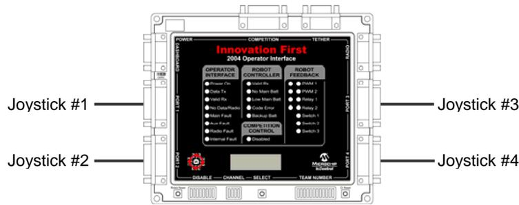
**Figure 4.3.1: Operator Interface with Four Joysticks**
