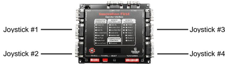
Figure 4.3.1: Operator Interface with Four Joysticks
