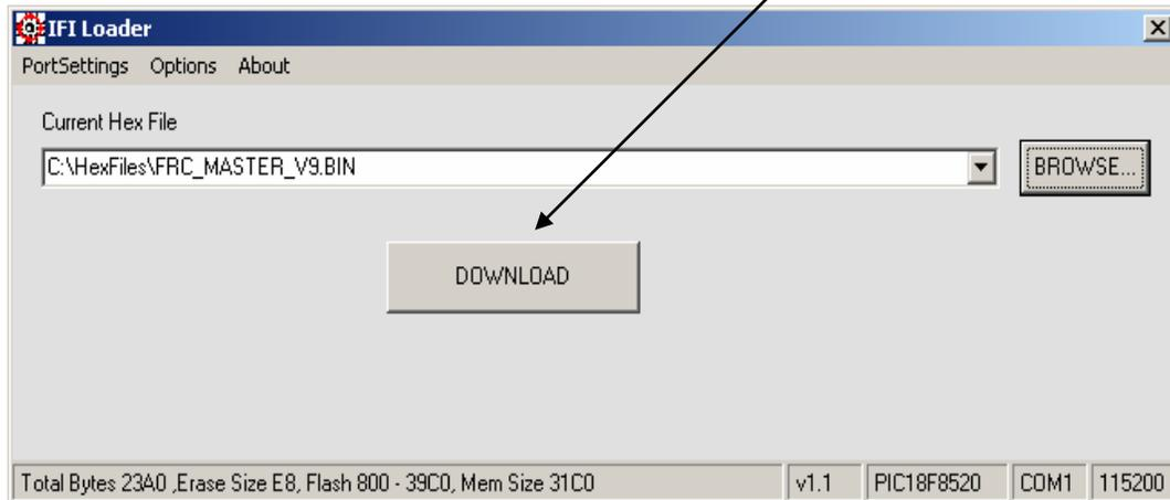
The **3rd Step** is to download the user code. Once the master firmware has been updated, the user code **must be reloaded**. In order to do this, repeat **Step 2**. Rather than selecting 'Master Files (\*.BIN)', you must select the 'INHEX32 Files (\*.HEX)' option. After downloading the appropriate user code (file), the robot controller is ready for use.
