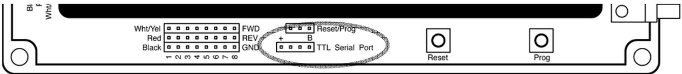
TTL Serial Port Pin-out
