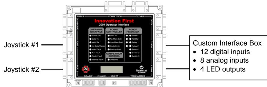
**Figure 4.3.2: Operator Interface with Two Joysticks and a User Box**
