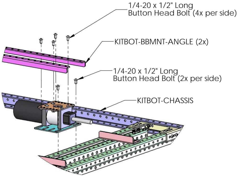
Attach Transmission Assembly to Kitbot Chassis in desired location using (2x) 1/4-20 Screws and Keps nuts per side.
