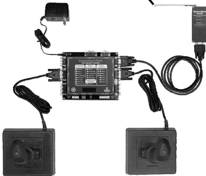
**Operator Interface with External Radio,
