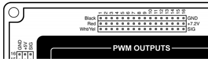
**Warning: The PWM outputs are only to be used with Victor/Thor 88x series Speed Controllers or servos. The use of other speed controllers may damage the unit and will void the warranty.**
