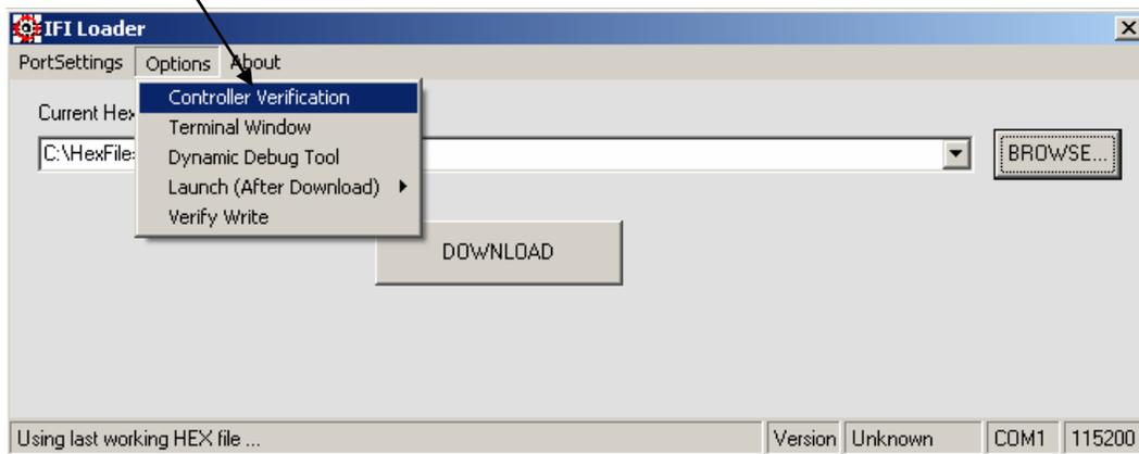
Now you should see 'Controller verification complete ...' on the lower left and 'FRC' in the lower right of the status window.
