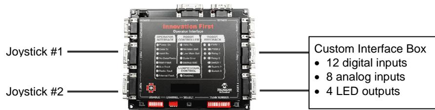
Figure 4.3.2: Operator Interface with Two Joysticks and a User Box
