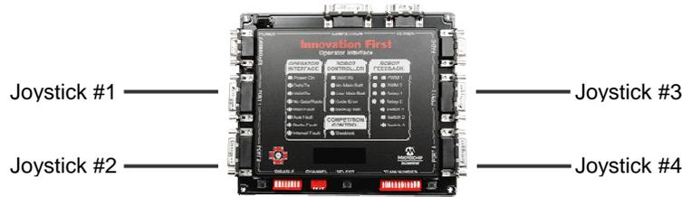
Figure 4.3.1: Operator Interface with Four Joysticks
