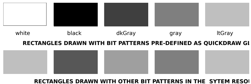
FIG 7 - RECTANGLES DRAWN USING BIT PATTERNS IN THE SYSTEM RESOURCE FILE
