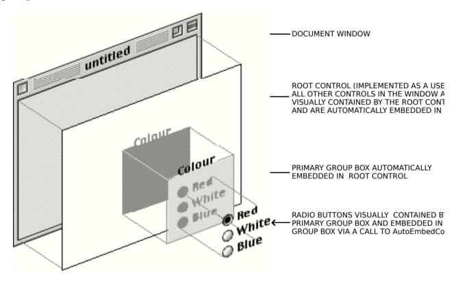
FIG 3 - THE ROOT CONTROL AND EMBEDDED CONTROLS
