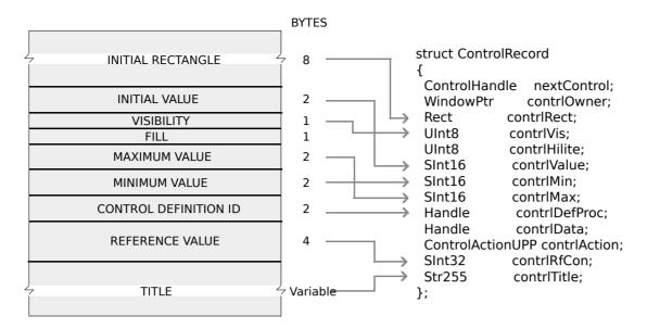
FIG 4 - STRUCTURE OF A COMPILED CONTROL ('CNTL') RESOURCE
