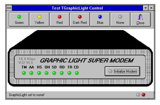
Other uses of GrafLight could include displaying modem-like lights on a status line for programs that use modem communications components. The GrafLites in the above form are the modem indicator lights and the two lights on the statusbar. Run the Testlite demo program to see how the lights work.
