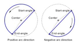
The eventual appearance of the circular segment is shown during its entry and changes immediately if the arc direction is changed during entry.
