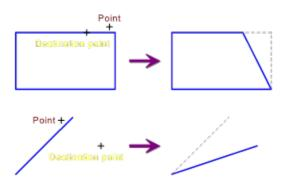
Altering the half-axes of ellipses or ellipse parts and moving the start or end angle of circle or ellipse parts (see graphic).
