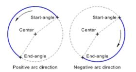
The appearance of the arc is show while it is being entered and changes immediately if the current arc direction is changed.
