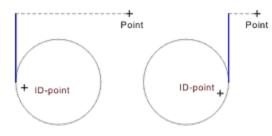
After identifying the object, a straight line appears which runs vertically and is tangent to the identified object.
