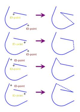
If the duplicate function was active while selecting the second object (e.g. because the CTRL key was held down), the identified objects remain intact. Otherwise they are deleted and only the new, extended curve remains.
