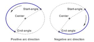
The later appearance of the elliptical arc is shown during entry and changes immediately if the current arc direction is changed during entry.
