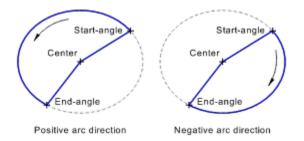
The later appearance of the elliptical sector is shown during its entry and changes immediately if the current arc direction is changed during entry.
