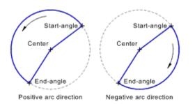
The sector's final appearance is shown during entry and changes immediately if the arc direction is changed during entry.
