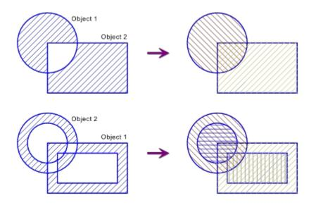
The areas of the objects which are shown hatched, are hatched or filled when the corresponding object is hatched or filled.
