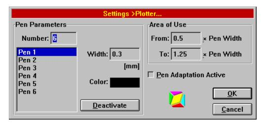
**Important!** Before you alter the settings in this dialog, it is *essential* that you read the section on <u>Notes</u> <u>on Plotter Output</u> fully. It contains important information on the correct use of plotters.
