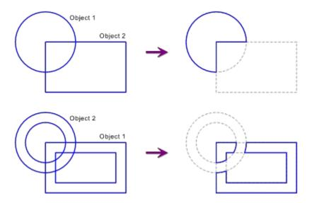
Note that the order in which the objects are identified is important. The last identified object is always "subtracted" from the object identified first.
