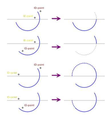
Note a basic rule for trimming: The object changes, wherever it is clicked on.
