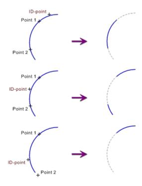
Note a basic rule for trimming: the object is always changed where it is clicked on! If both points lie outside the object outline, an error message appears. **Note:** If a non-standard object (e.g. a surface or a curve) is to be trimmed, it must be resolved to its constituent parts first using the command <u>Trim Object>Resolve Completely</u>. These can then be trimmed.
