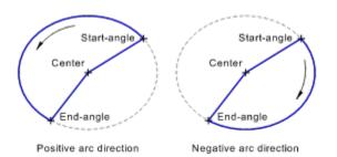
The later appearance of the elliptical sector is shown during entry and changes immediately if the current arc direction is changed during entry.
