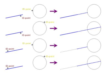
Note a basic rule for trimming: The object changes, wherever it is clicked on.
