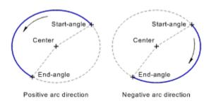
The later appearance of the elliptical arc is shown during entry and changes immediately if the current arc direction is changed during entry.
