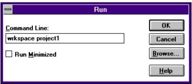
From the Program Manager's Run dialog box (or other equivalent Windows command line), run WorkSpace with a command line argument specifying the group to launch. The format is: **[path]wrkspace [group name]**. If \*.wsp files are associated to WorkSpace, just the filename of the group can be used.
