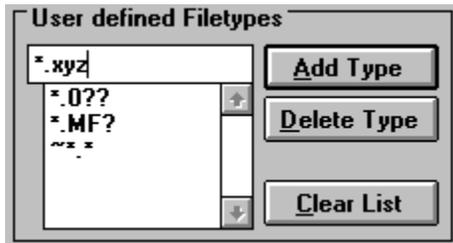
As you can see in the picture, the user has entered the new filetype "\*.xyz" in the text field of the combo box. By pressing the "Add Type" button, the new filetype will be added to the list of user defined filetypes shown in the list. If you select a filetype in the list, it can be deleted by pressing the button "Delete Type". Please note, that there is no confirmation for that deletion. If you press the button "Clear List", the list will be completely deleted after a confirmation.
