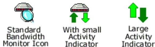
The Activity Indicator works like a Network LED. When there is activity on the selected Network Card, one of the two LEDs (Upload/Download) is activated.
