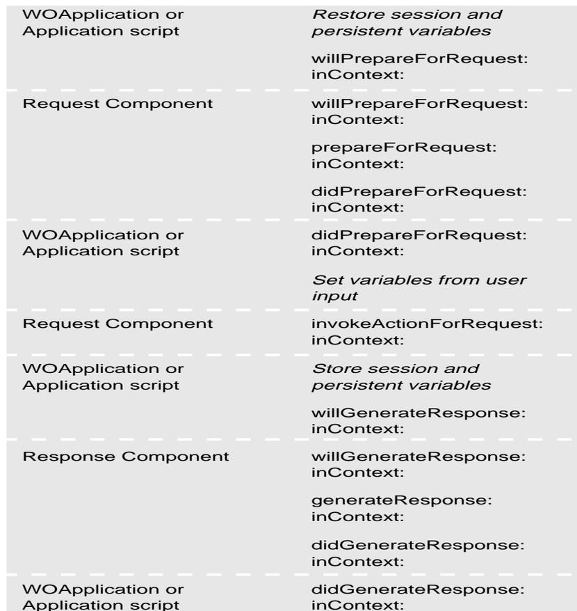
Figure 2. The Sequence of Events in One Cycle of the Request-Response Loop
