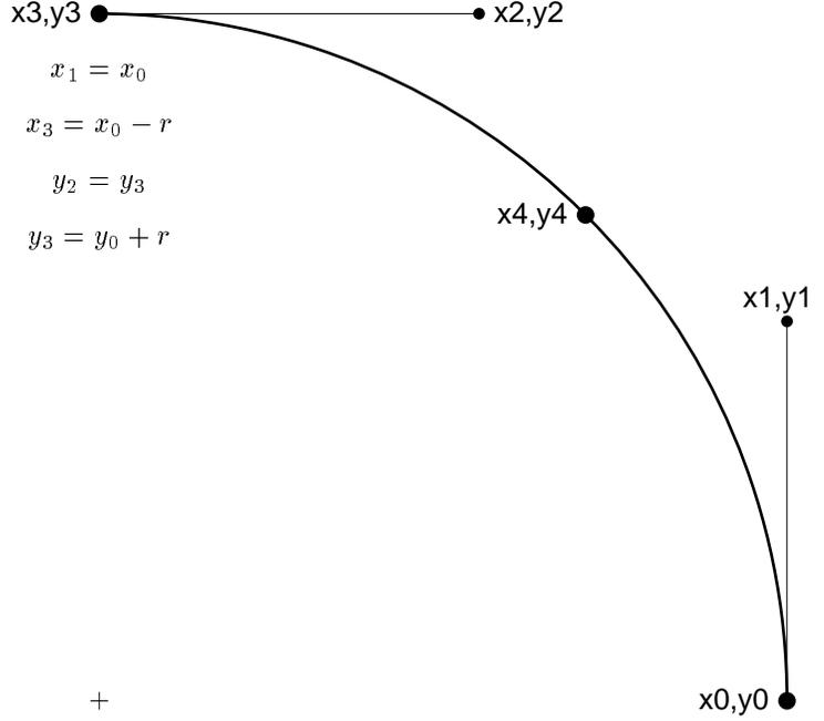
$$\begin{aligned}x_1 &= x_0 \\x_3 &= x_0 - r \\y_2 &= y_3 \\y_3 &= y_0 + r\end{aligned}$$
