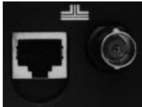
Regardless of the Ethernet cable option you choose, adding a NeXT computer to the network is a simple task: simply connect the computer to the network and turn it on. NeXTstep<sup>™</sup> automatically senses which type of Ethernet wiring you have used and correctly configures itself. It's that easy.
