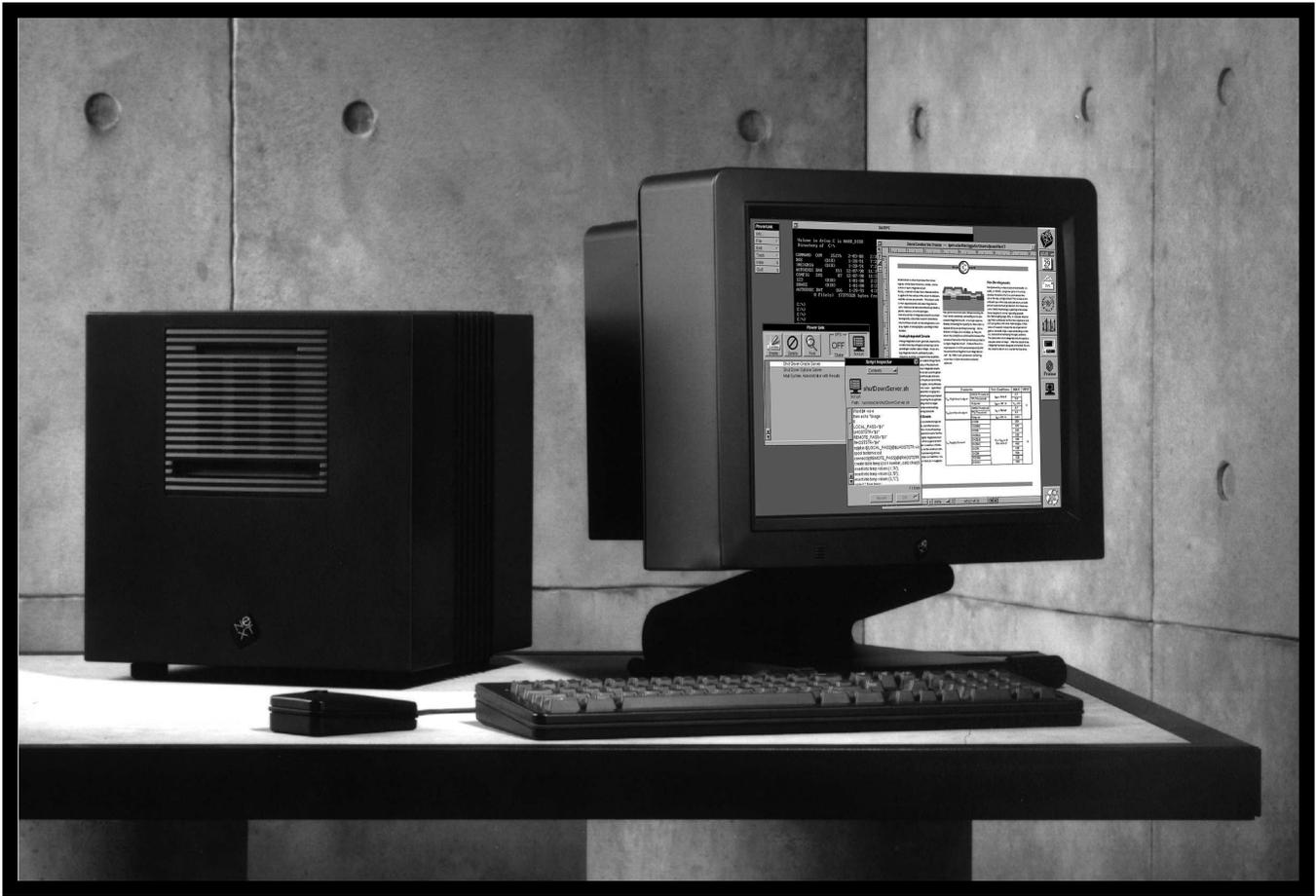
*The NeXTcube is a versatile, easy-to-use workstation that can be utilized as a desktop monochrome system, true color 32-bit-perpixel color/video workstation or file server system, all featuring NeXT's object-oriented operating and development environment.*
