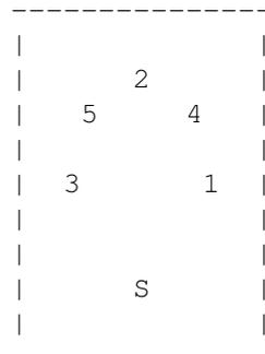
S = Shield of the Plug (must be connected to Pin 2)
