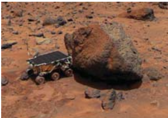
Figure 3.33 A close-up of the Sojourner rover taken during the Mars Pathfinder mission in 1997 as it placed its alpha proton X-ray spectrometer (APXS) upon the surface of the rock 'Yogi' to determine its composition. (The rover is about the size of a microwave oven.) Results show this rock has a composition similar to common basalts found on Earth.
