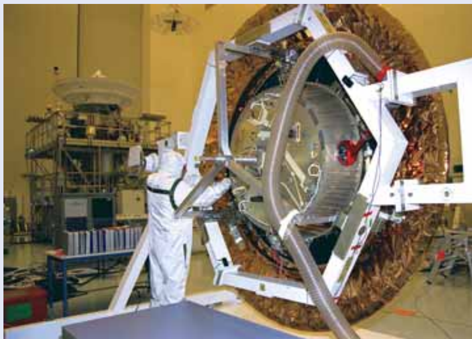
Figure 5.13 The Huygens Probe during final assembly. The 2.7 m front shield is clearly visible.
