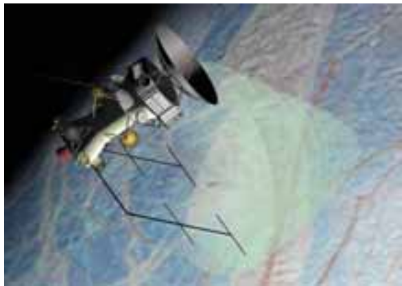
Figure 4.28 A Europa orbiter in action (not JIMO, but a simpler mission that has now been cancelled). The blue beam illuminating the surface is a schematic indication of the ice-penetrating radar beam, which is intended to map the ice thickness with a depth resolution of about 100 m.
