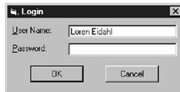
To create the logon screen, start a new project in Visual Basic. Add controls to a standard form so that it is similar to Figure B4.2. After completion of the logon form, you can begin entering the code.
